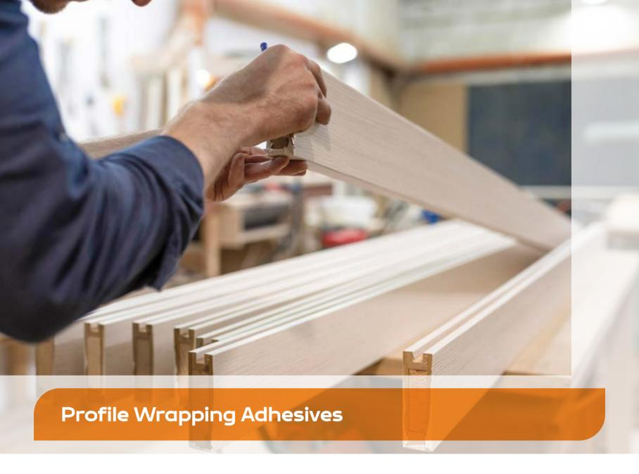
In the furniture industry, profile wrapping is a well-established application for surface treatment of components such as furniture parts, skirting boards, wall and ceiling panels, door components, and various other profiles. A wide selection of materials can be used for profile wrapping, including thermoplastic foils (PVC, PP, PET), paper, veneer, and CPL/HPL.
